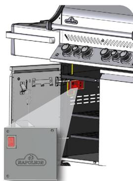
Turn the Power Switch ON located on the box inside the grill cabinet.
