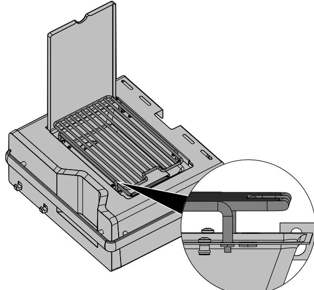
**Cooking Grid Placement:** The cooking grid can be placed at two different heights. The lower height is for use with pots or pans. The higher position is to be used when searing meats. Ensure the burner is off and the grid is cool to the touch before changing between the two heights. The grid must be at the lower height in order to close the lid.
