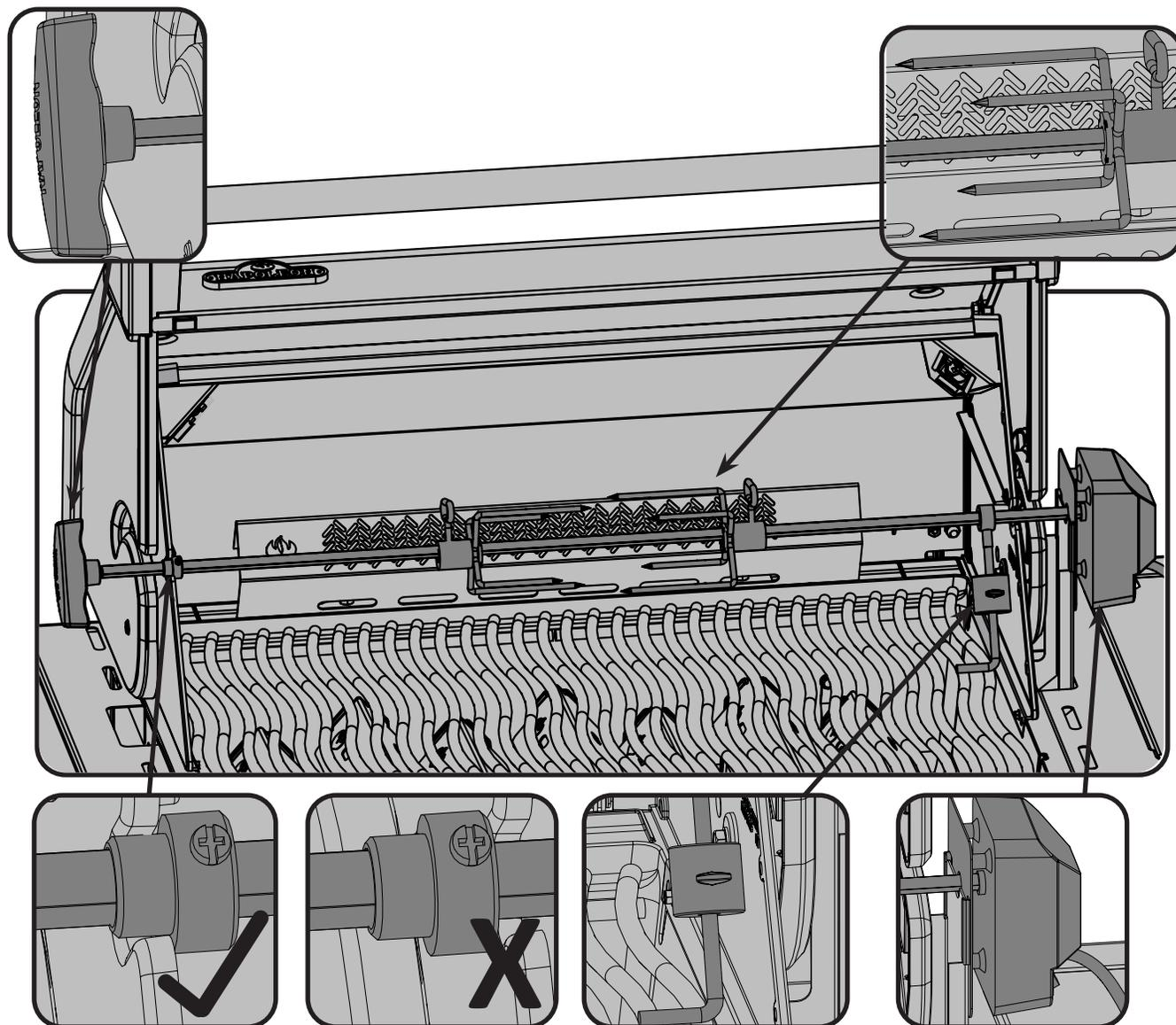
Ensure stop bushing is tightened on the inside of hood casting.
