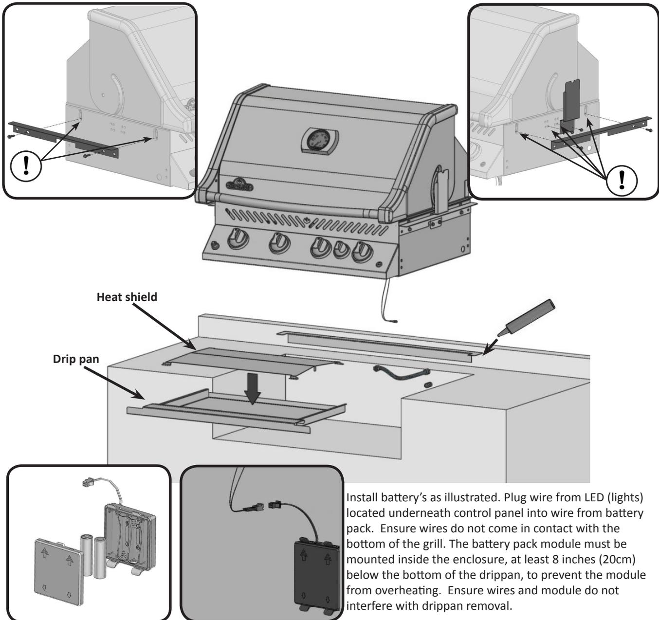
Install battery's as illustrated. Plug wire from LED (lights) located underneath control panel into wire from battery pack. Ensure wires do not come in contact with the bottom of the grill. The battery pack module must be mounted inside the enclosure, at least 8 inches (20cm) below the bottom of the drippan, to prevent the module from overheating. Ensure wires and module do not interfere with drippan removal.
