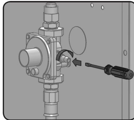
This unit includes an internal regulator which stabilizes the gas pressure and improves grill performance. This regulator cannot be adjusted. There is a pressure tap located on the side of the regulator. It can be used by a qualified service person when servicing the grill to determine if the regulator is functioning properly. The screw within the pressure tap must always be kept tight, except when performing a pressure test on the regulator (qualified service personnel only).
