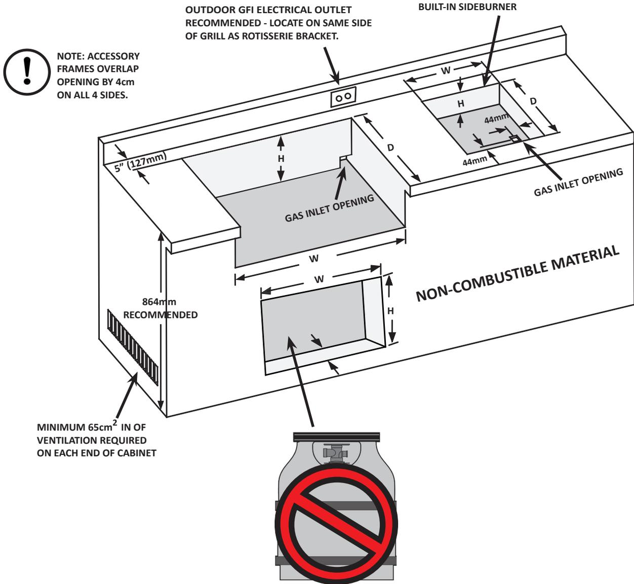
**WARNING!** CABINET FRAME, CABINET AND COUNTER TOP MUST BE MADE FROM NON-COMBUSTIBLE MATERIAL.
